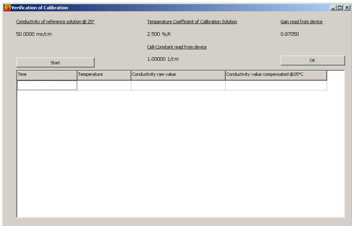
After verification of the current calibration settings you may press the button "OK". This will stop the online measuring procedure and a final information window will be displayed.
