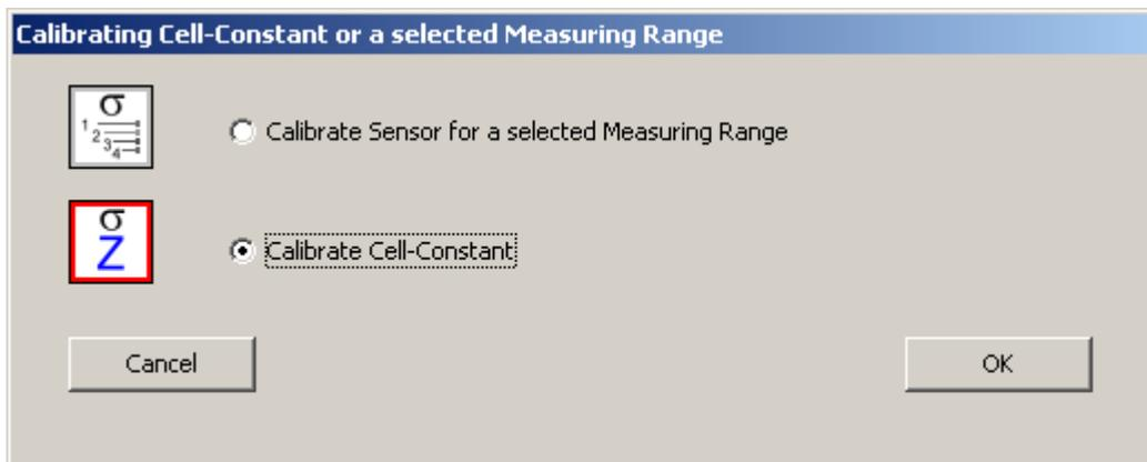
Pressing the button "OK" will initialize all gain or correction factors from measuring range 1 to 4 with a value of 1.0.
