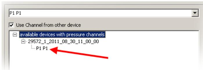
The list of water level calculations indicates that a valid second channel has been assigned to the calculation rule.
