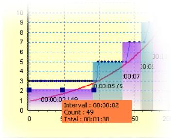
A floating panel indicates the interval, measurements count and total measuring time, if a column is selected and resized.
