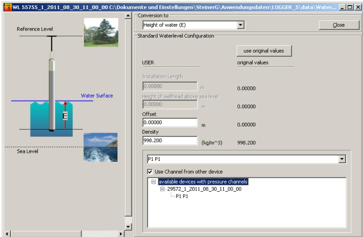
On the bottom right corner a tree view listing all available or currently loaded files allows to select any desired pressure channel. The checkbox "Use Channel from other device" is activated. You need to tell the Viewer from which device or file the barometric pressure should be derived from for water level calculation.
