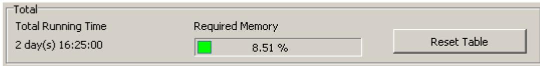
If the total required memory exceeds 100% of device memory capacity, the memory gauge indicator changes the color from green to red.
