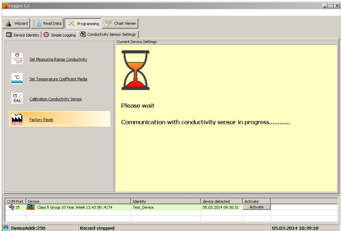
When initialization has been completed, the information panel will disappear and the "Current Device Settings" show the default values for all settings of the conductivity sensor.
