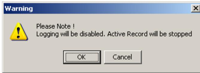
You can proceed by pressing the "OK" button which will stop a running record. The selected measuring range then becomes activated. The application confirms the successful change of measuring range by hiding the "Write" button in the left lower corner of the dialog window. Simultaneously the new selected measuring range will be displayed on the main form as shown in the picture below:
