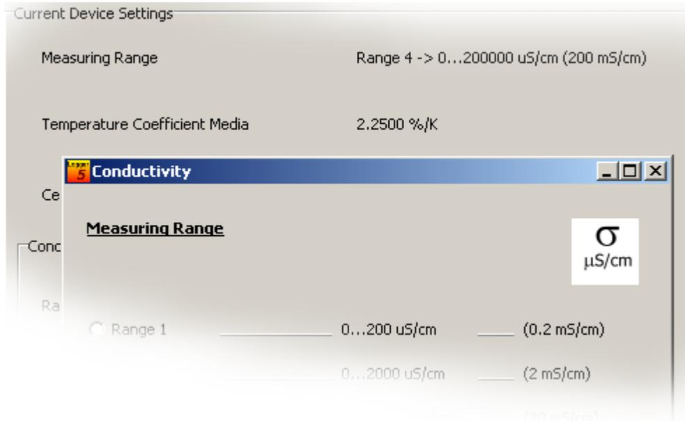
You may also select the tab sheet "Conductivity Sensor Settings" where you can find a possibility to select measuring range of the conductivity sensor.
