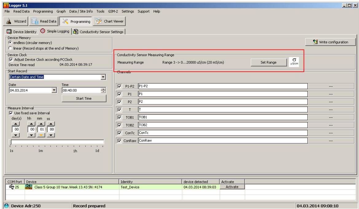
The conductivity sensor provides the following measuring ranges:
