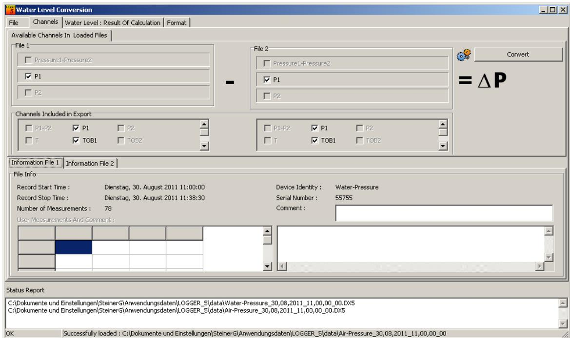
The Water Level Converter selects the P1 channel from each file. In the example all available raw data channels are selected as well.
