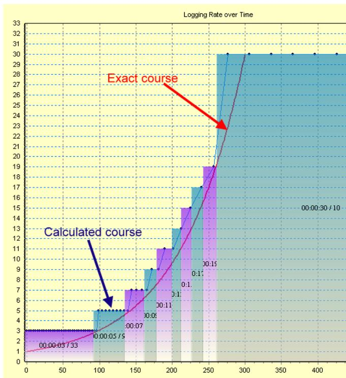
Each section of the semi-transparent column chart can be adjusted with the mouse. You can change interval and count by changing the size of a column.
