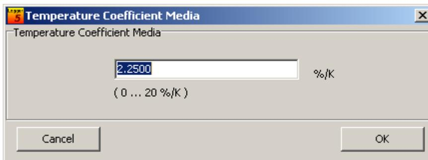
Proceed with the button "OK" to confirm new value for the temperature coefficient. Pressing "Cancel" will not store the value. Anyway you will need to check the programmed logging regime and to start a new record.
