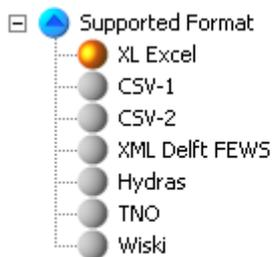
The text converter tool converts the original data stored in the \*.DX5 file format into several ASCII file formats to export measuring data for other applications.
