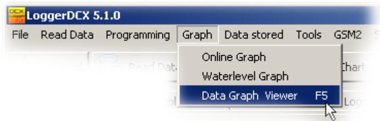
The Viewer Chart tool allows users to view measuring data, including several files at the same time. The measuring data can come from the same device or you may inspect data retrieved from different logger devices.
