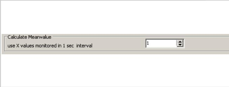
This function enables the averaging over "X" measurements at intervals of one second each. Recording is initiated only after the average has been determined, even if the recording interval chosen is smaller.
