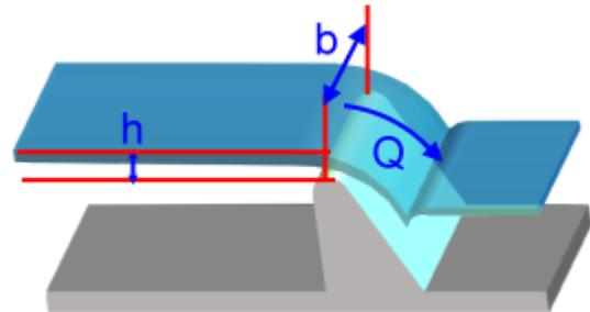
$\mu$  represents the overfall coefficient. This coefficient is dimensionless and depends on threshold shape and partially on the head on weir
