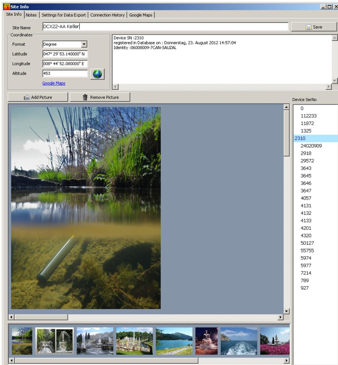
The "Site Info" maintains additional information concerning the measuring station where the logger device is located in the field.
