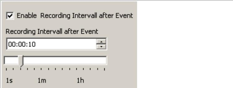
Recording is done at a fixed interval independent of Fixed Save-Interval. If Recording interval after event has been selected in addition to Event Detect Interval, the smaller of the two intervals applies.
