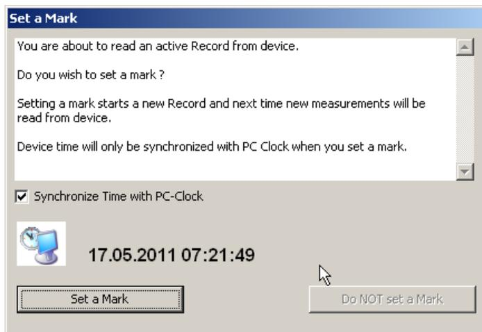
Leaving the check box "Synchronize Time with PC-Clock" enabled and pressing "Set a Mark" the time on the device will be adjusted to the time of the PC-Clock and a new record will be started. The start time of the new record will be set such that the logger will maintain the assigned measuring interval. A new record will appear now as first item in the table of content showing the record structure - please refer to [Reading data from connected device Part 1](#)
