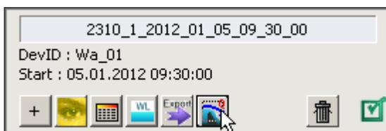
Press the tool button with the overfall icon
