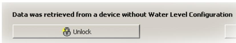
The user now may edit manually "Installation length", "Height above sea level", "Offset" and "Density" and select one of the available calculation methods.
