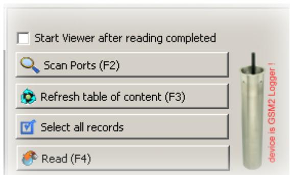
On the bottom of the window the GSM-2 unit appears in the device list.
