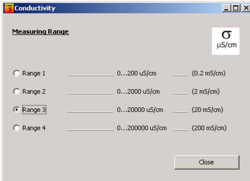
Selecting a different measuring range than currently activated, a button "Write" will become visible.
