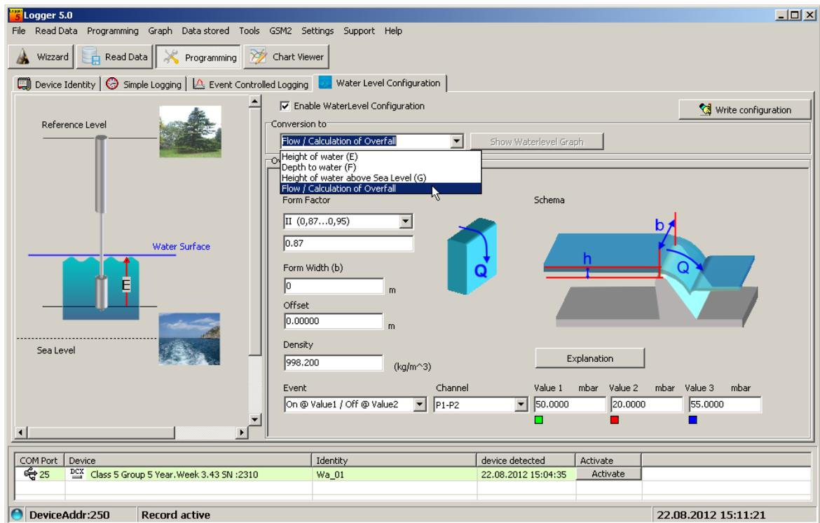
The programming of the logger device for such applications is presumably combined with event controlled monitoring. See also [Programming Event Controlled Logging](#)
