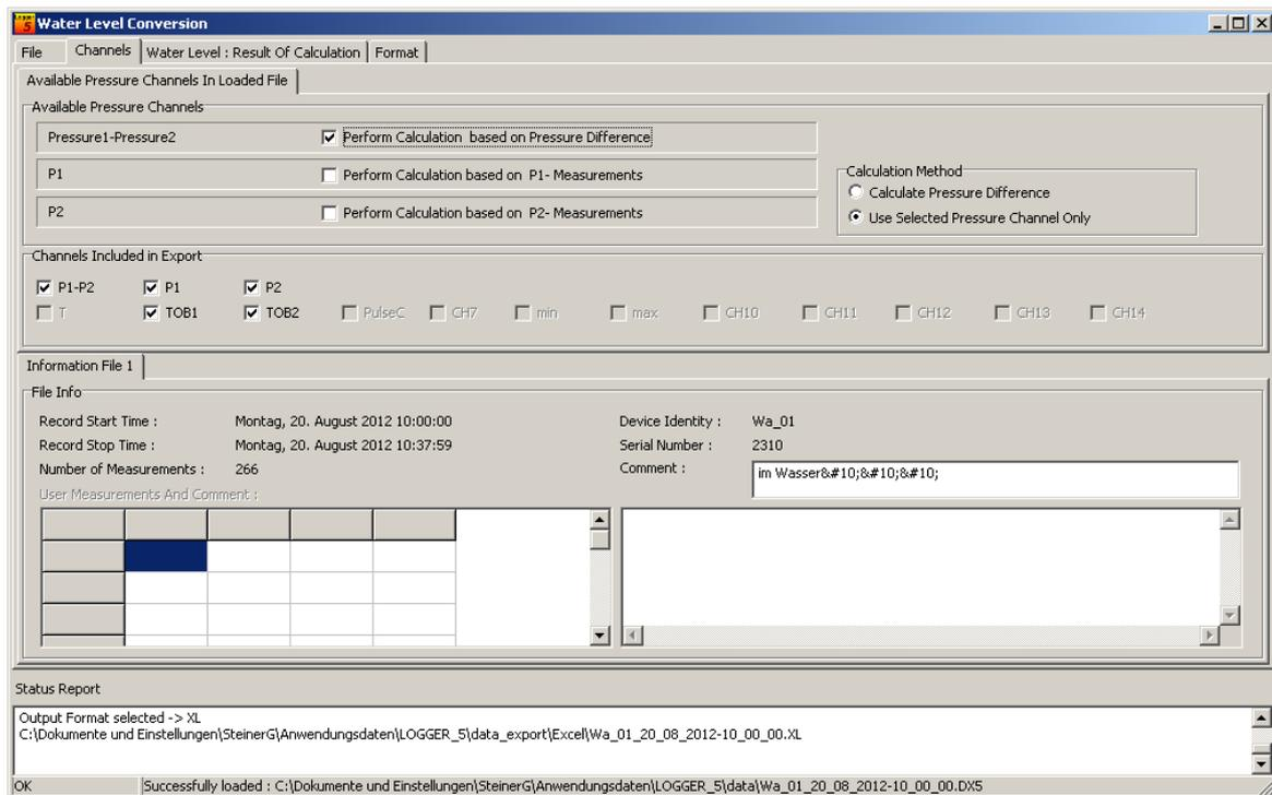
This is a meaningful pre-selection because the P1-P2 channel is available for the DCX-22 AA logger device only. You may find further information about the DCX-22 AA in section [About Waterlevel and Pressure](#) .
