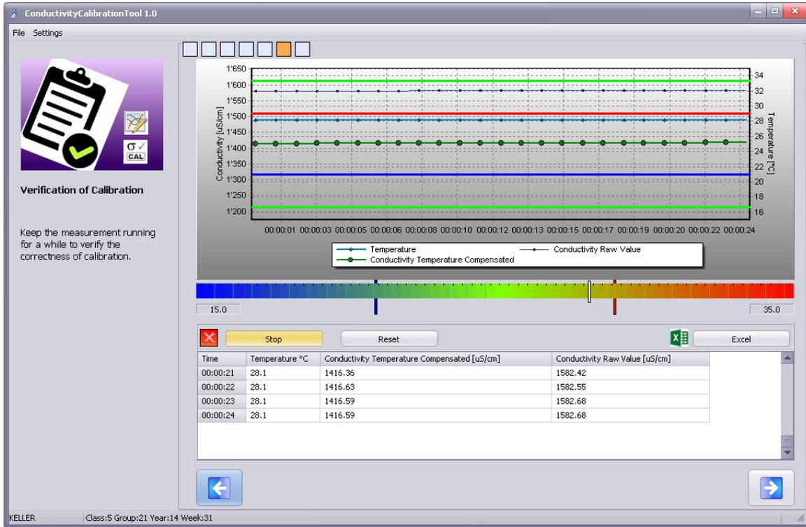
After finishing the calibration, the temperature gradient of the liquid used to measure should be recorded and written on the probe. Now the probe is ready for measurement in field applications. Temperature coefficient is only required for linear compensation, but to finish the program the button “write Temperature Coefficient” should be pressed. Afterwards it is possible to set the device to SDI-12 Mode if needed.
